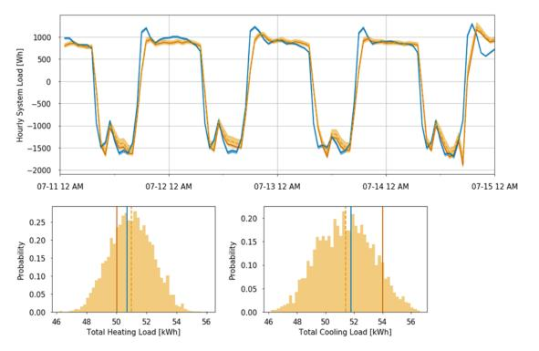
Experimental results and models (including uncertainty) for a BESTEST 940 like case with high thermal mass and solar loading. Top plot is hourly data with heating being positive and bottom plots are cumulative heating and cooling loads.
